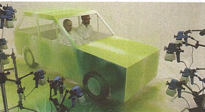
Semi Automatic Painting Machine, 2014
